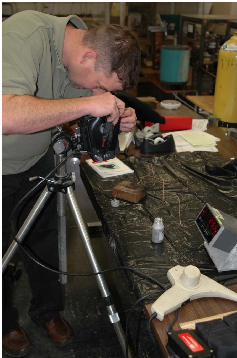
Figure 25. This picture shows how we recorded the temperature of the eutectic with a thermocouple and calibrated the infrared camera by adjusting the emissivity setting until the temperature shown on the camera matched the temperature on the thermocouple.
