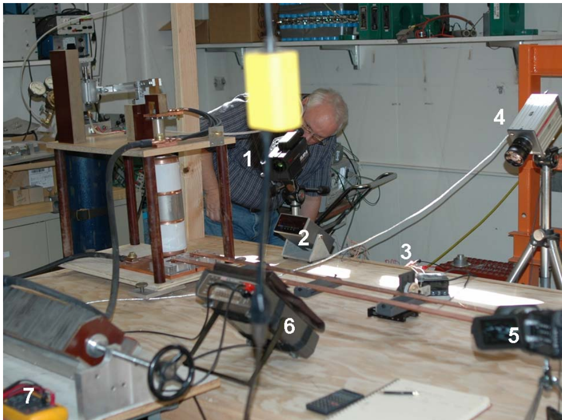
Figure 26. This photograph shows how we positioned many of the sensors in this experiment. Going clockwise from our technician on the infra red camera we have the IR camera on a tripod (1), the thermocouple meter (2), micro-strain meter and the load cell on the table (3), the high speed camera on a second tripod (4), the high definition camera on the short tripod (5), the micro-ohm meter on the table (6), and the fluke meter on the battery cart (7). Not pictured are three other load cells, an oscilloscope, and a digital camera for still photos. (The “yellow box” is not part of the experiment – just an out-of-control power cord)
