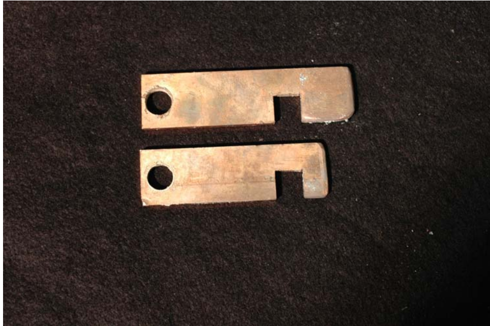
Figure 11. The notch in the bar was centered over the end-cap of the eutectic pool. By varying the position of the notch relative to the end of the bar we could vary the power-bar to gun-bar separation
