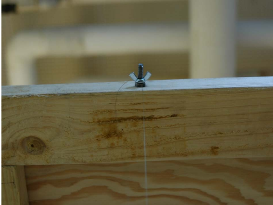
Figure 20. The aspect shown here is the chamfered edge of the rail support looking up at the all-thread rod where the monofilament line is squeezed between the two nuts. The advantage of this system allowed for continuous “tweaking” of the pendulum as we sought to have consistent tension on all lines and a square and level presentation of the rails to the eutectic and the load cells.
