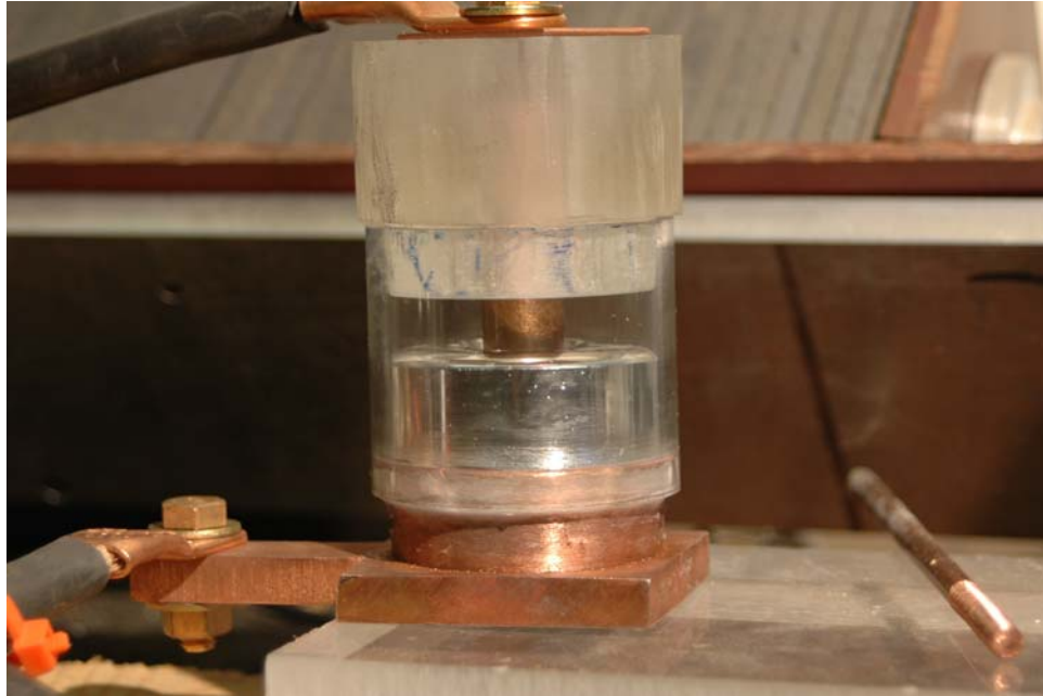
Figure 9. This is a profile view of the polycarbonate cylinder filled with the eutectic and the wetted copper rod. By swapping the terminals we were able to observe consistent fluid behavior regardless of the direction of the current flow.
